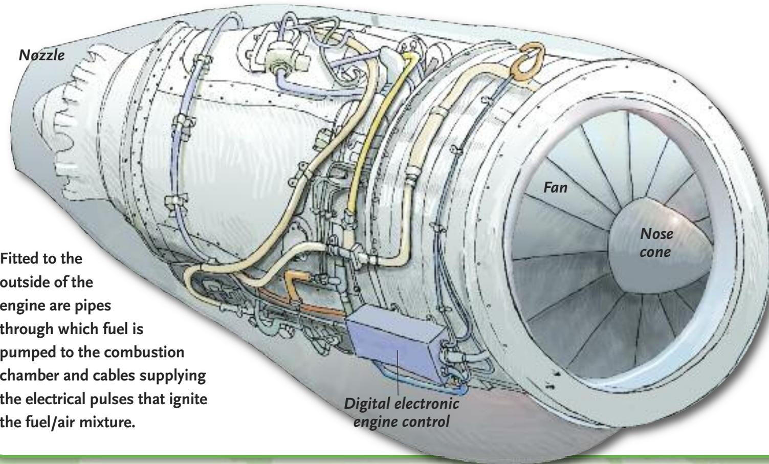
Fitted to the outside of the engine are pipes through which fuel is pumped to the combustion chamber and cables supplying the electrical pulses that ignite the fuel/air mixture.
