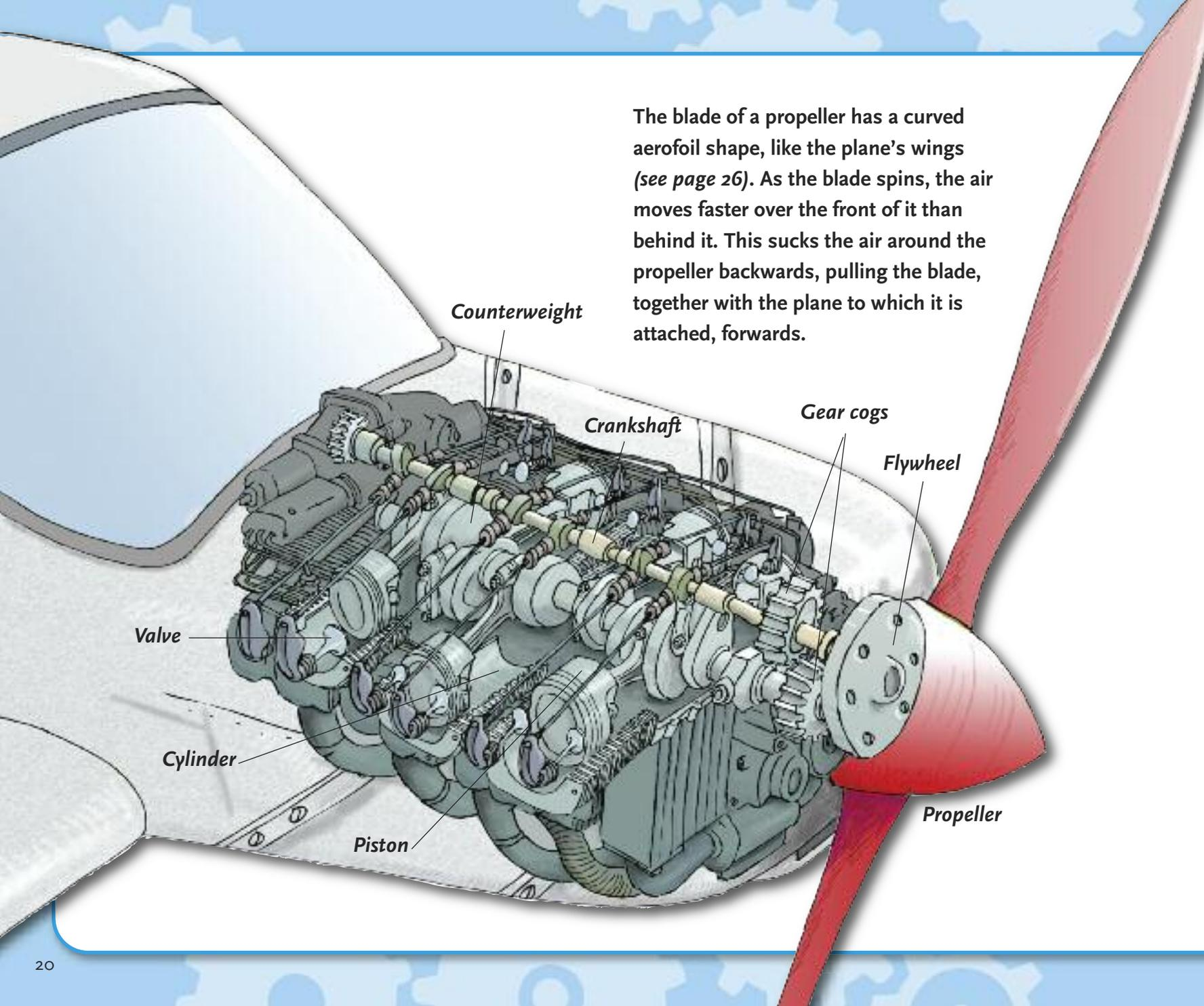
The blade of a propeller has a curved aerofoil shape, like the plane's wings (see page 26). As the blade spins, the air moves faster over the front of it than behind it. This sucks the air around the propeller backwards, pulling the blade, together with the plane to which it is attached, forwards.
