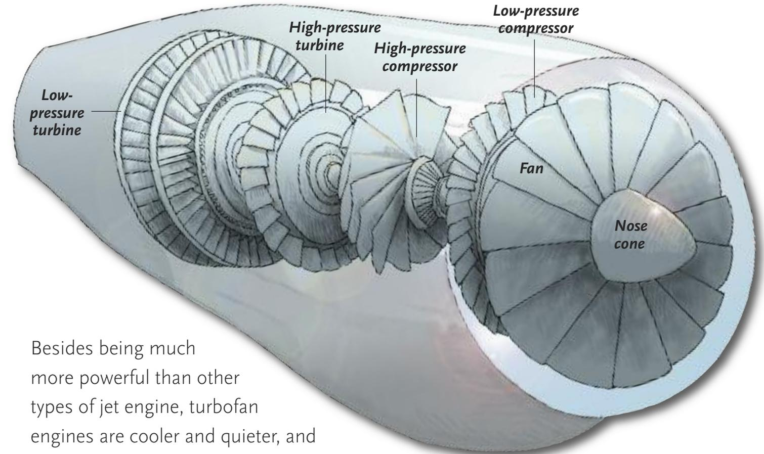
Besides being much more powerful than other types of jet engine, turboprop engines are cooler and quieter, and more economical in their use of fuel. They are also equipped with thrust reversers. When in use, the jet of hot exhaust gases is deflected forwards instead of backwards, producing a force which rapidly slows down the plane landing on the runway.
