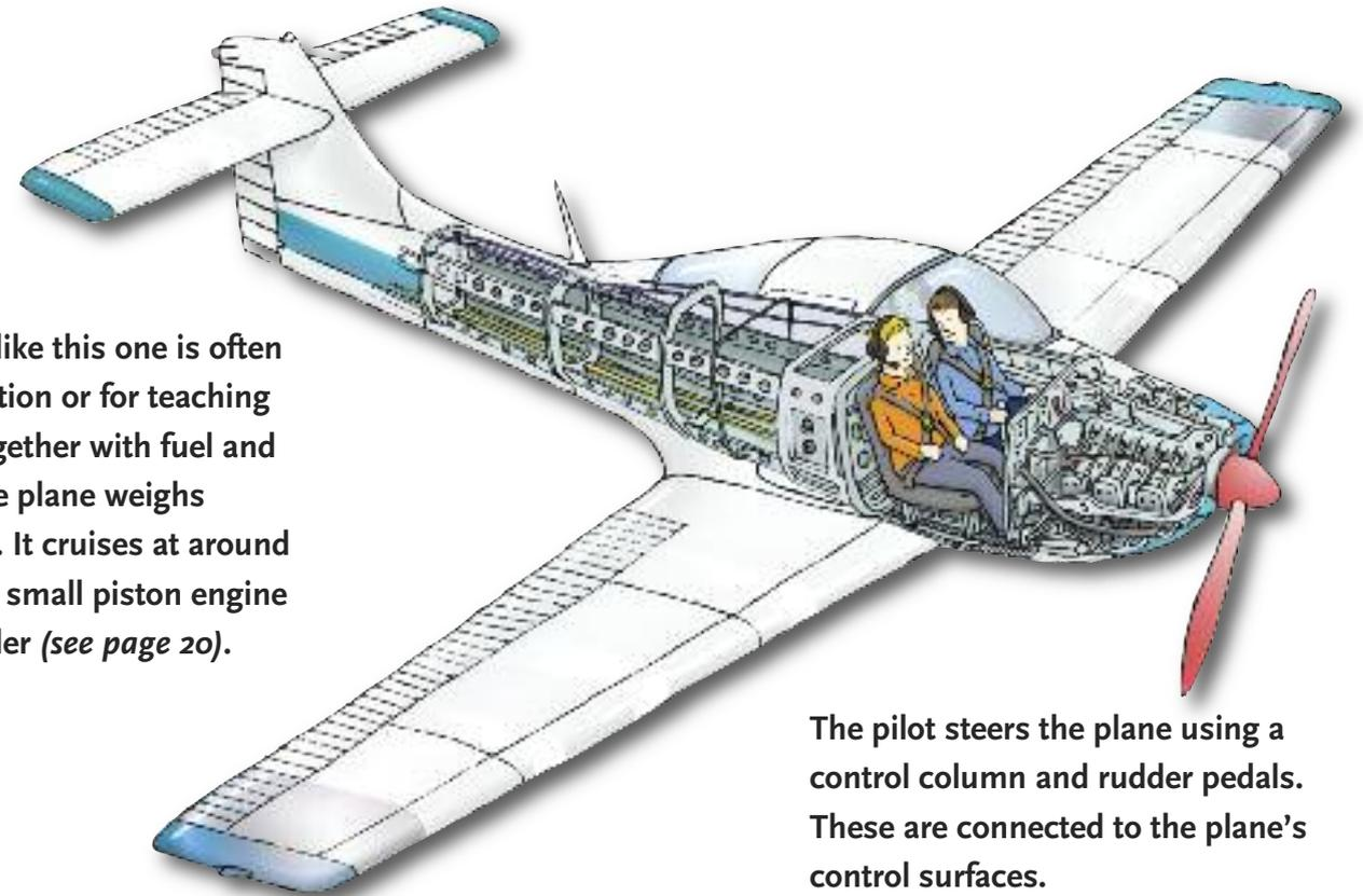
**A light aircraft like this one is often used for recreation or for teaching pilots to fly. Together with fuel and passengers, the plane weighs around 600 kg. It cruises at around 200 km/h. The small piston engine drives a propeller (see page 20).**
