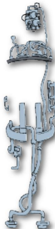
**LANDING GEAR** During flight, the wheels are folded up into the nose and undersides of each wing.
