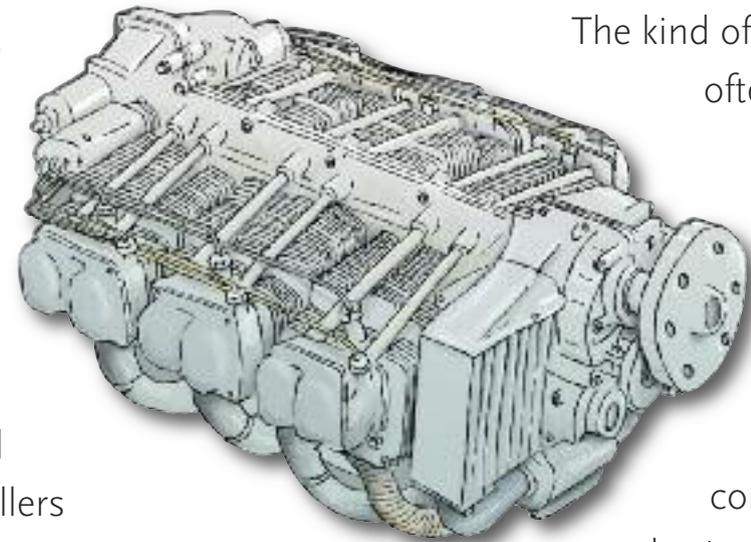
The kind of piston engine most often used in a light aircraft is called a flat engine. It has two banks of cylinders opposite one another. The pistons are connected to a horizontal crankshaft.
