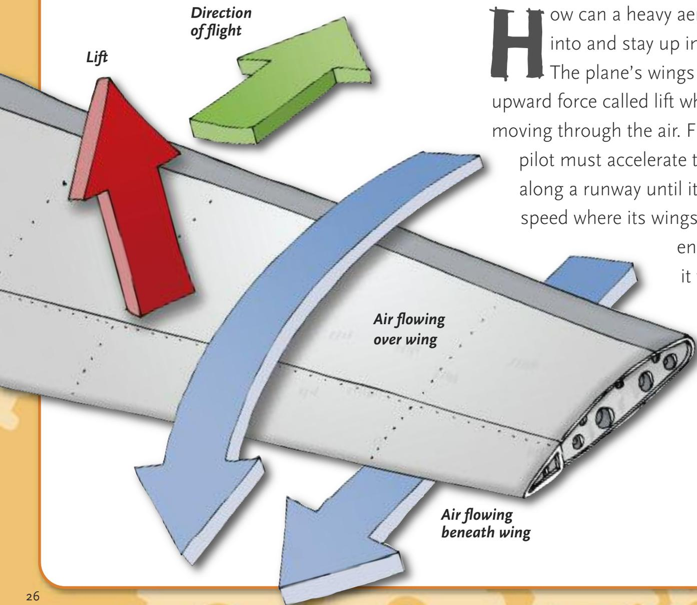
**H**ow can a heavy aeroplane rise into and stay up in the air? The plane's wings provide an upward force called lift while it is moving through the air. First, the pilot must accelerate the plane along a runway until it reaches the speed where its wings provide enough lift for it to take off.
