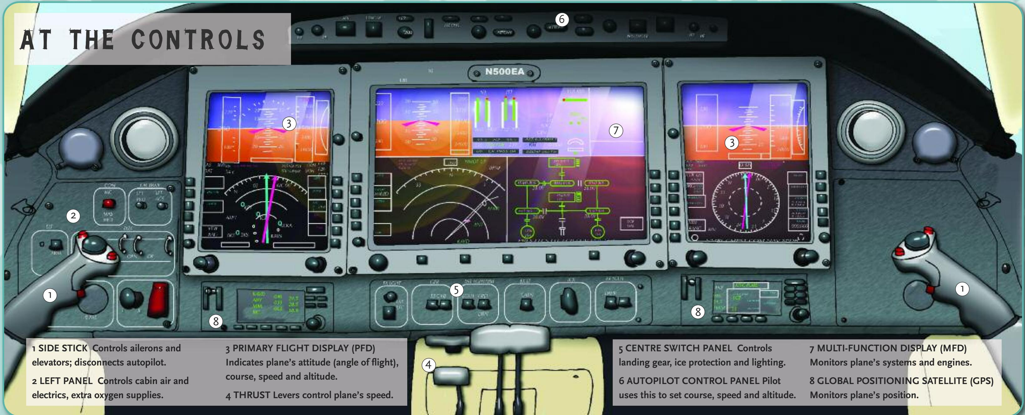
**1 SIDE STICK** Controls ailerons and elevators; disconnects autopilot.
