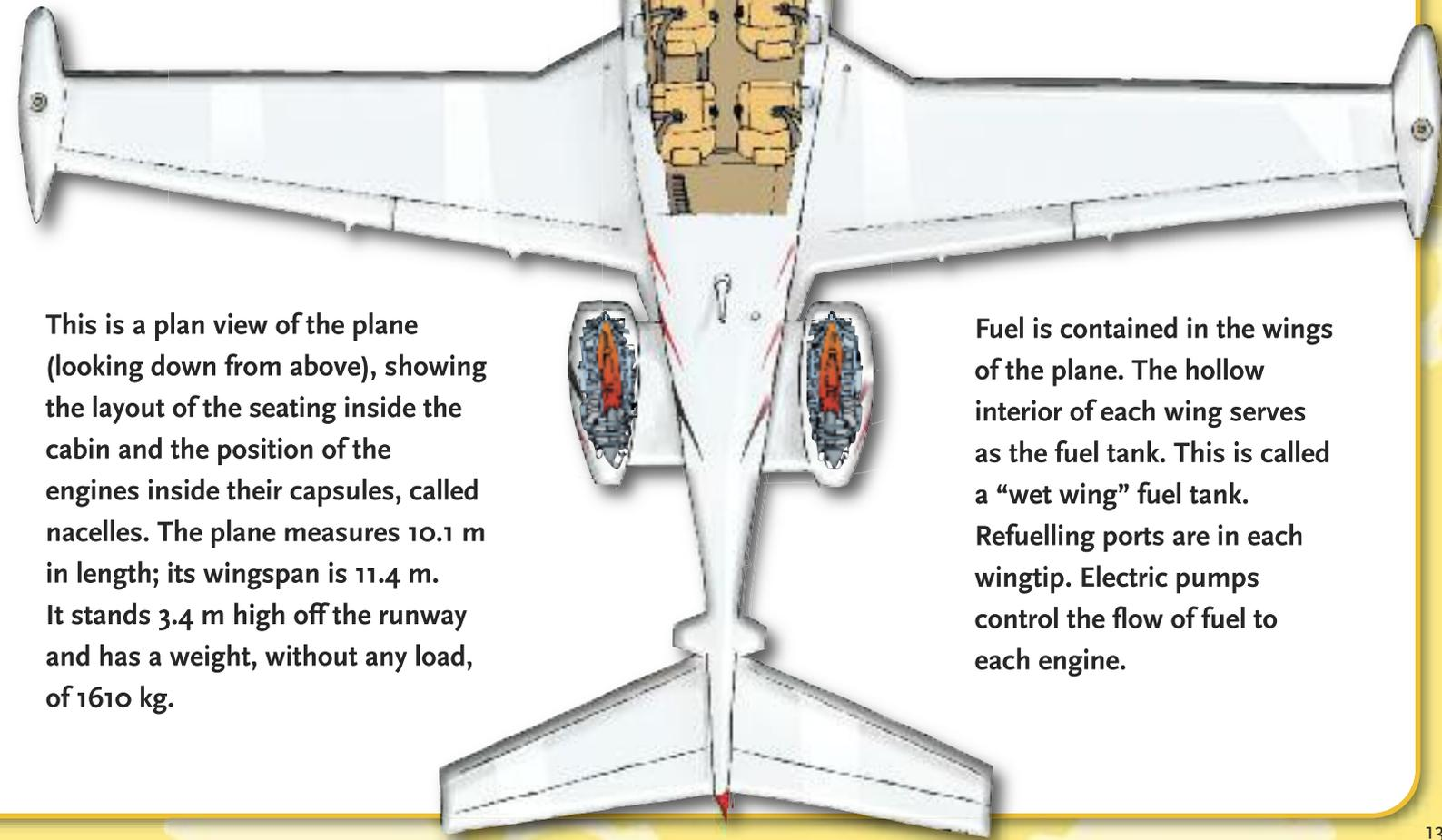
This is a plan view of the plane (looking down from above), showing the layout of the seating inside the cabin and the position of the engines inside their capsules, called nacelles. The plane measures 10.1 m in length; its wingspan is 11.4 m. It stands 3.4 m high off the runway and has a weight, without any load, of 1610 kg.
