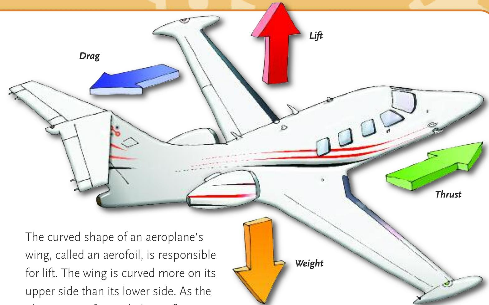
The curved shape of an aeroplane's wing, called an aerofoil, is responsible for lift. The wing is curved more on its upper side than its lower side. As the plane moves forward, the air flowing over it is made to move faster than the air flowing beneath it. The moving air creates less pressure on the upper side than on the lower side. An upward force, called lift, is the result.
