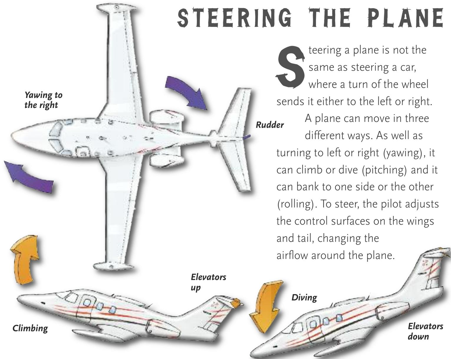
Swivelling the rudder on the tailfin pushes the nose left or right. Raising flaps on the tailplane, called elevators, causes the nose to rise and the plane to climb. Lowering them causes the nose to drop and the plane to dive.
