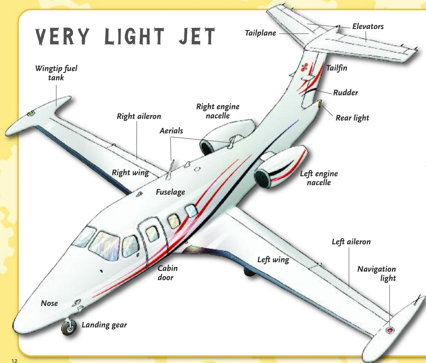
This is a type of plane called a Very Light Jet. Powered by two small jet engines, it is a six-seater that can be flown by a single pilot.
