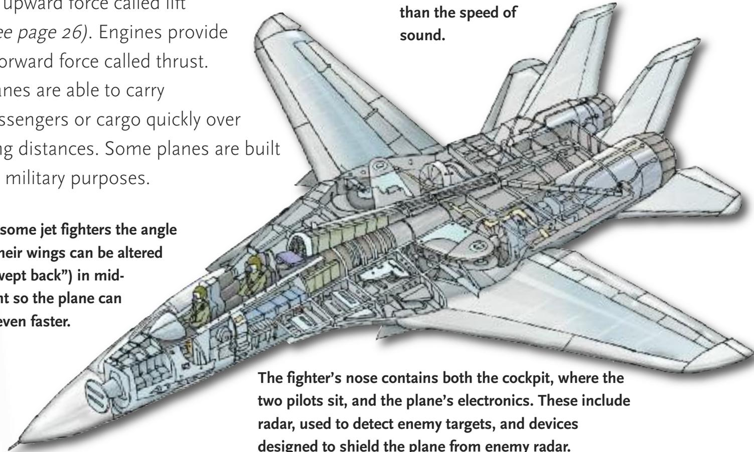
**The fighter's nose contains both the cockpit, where the two pilots sit, and the plane's electronics. These include radar, used to detect enemy targets, and devices designed to shield the plane from enemy radar.**
